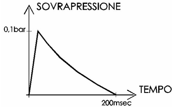
Figure 3. Overpressure versus time diagram
